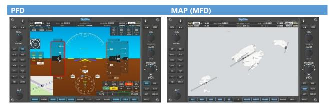
There is no real MFD in SkyElite but when PFD is set to MAP mode, it looks like a MFD. When SkyElite is used in two simultaneous screens, tablets or iPads, the use of MAP as PFD is highly recommended.
