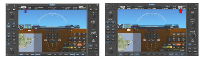
From version 1.2, Barometer value can be entered by virtual keyboard, by clicking or touching on it.
